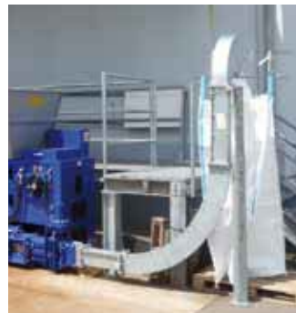
Discharging tunnel (optional)
