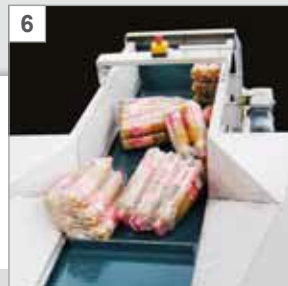
6 Conveyor Filled liquid containers are conveyed automatically from the funnel via the conveyor to the machine.
