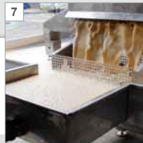
7 Separation of liquids Removement of liquids through a coarse filter box.
